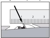
Figure 11. Correctly adjusted cutter.
